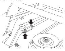
4 Screw out (extend) the stay to raise the rear edge of the cover. Screw in (shorten) the stay to lower the rear edge of the cover.
